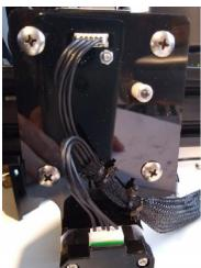
Laser side and jig mount point is the left hand side of this image. Note the top left screw is closer to the edge of the acrylic.
