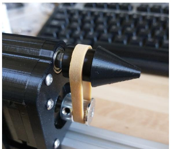
Screw the required end onto the tailstock, loosen the locknut and slide the tailstock up to secure your work.
