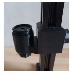
Attach the leg to the adapter using the supplied bolt. Probably best done with the leg at its lowest setting. (Photo of leg attached to the D1 Pro to follow<sup>©</sup>)
